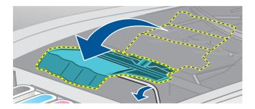
3 Pull the latch up and back to uncover the printheads.
